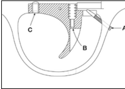
**Screw A:** Adjusts the second stage weight setting. To increase the weight, turn the screw anti-clockwise. To lighten the weight, turn the screw clockwise.
